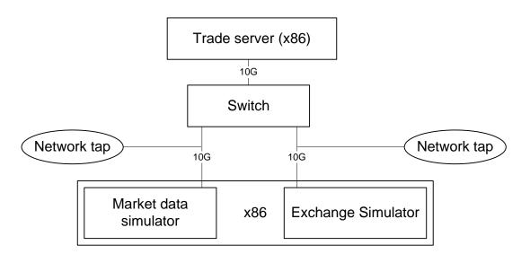
The x86 trade server (2x Intel Xeon E5-2690 @ 2.9GHz, with 192 GB of RAM) is a high end specification and has been optimised for low latency. The network cards implement kernelbypass, and various power and networking settings have been tweaked in the BIOS and elsewhere. (See the start of section 5, page 9 of the Finteligent report.)
